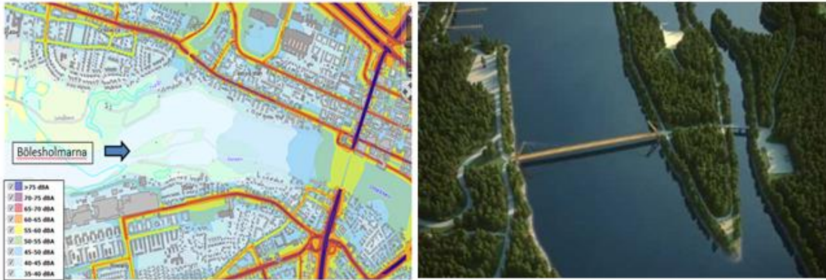
Figure 6C3 The equivalent sound level Leq\ 24h\ dB(A) at Bölesholmarna in Umeå river has been calculated in noise map below 35 dBA. To the right, an image of planned pedestrian bridge to Bölesholmarna in the city center at Umeå River.
